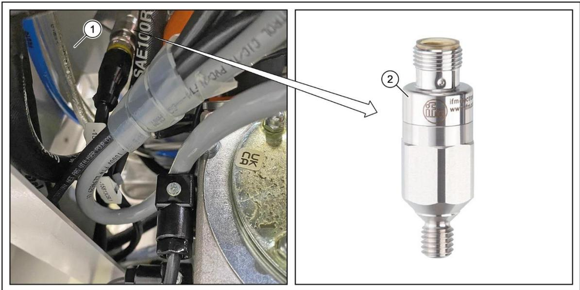
Fig. 110 Vibration sensor on the dolly - SynchroFine
