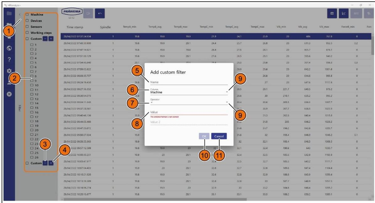
Fig. 80 Filter function - add filter menu window
