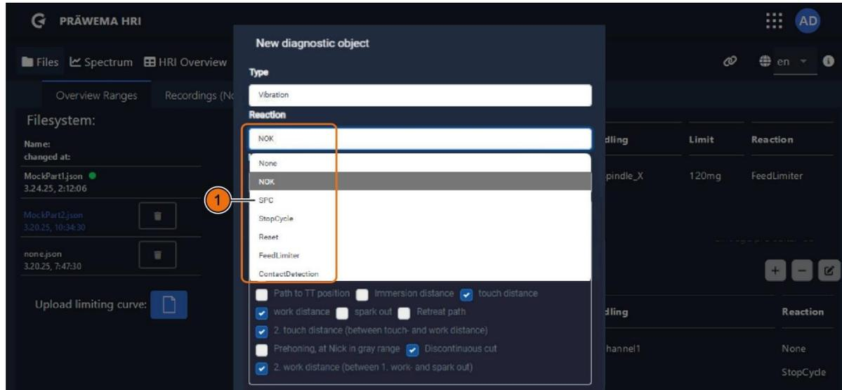
Fig. 16 New diagnostic object menu - selection list of Reactions
