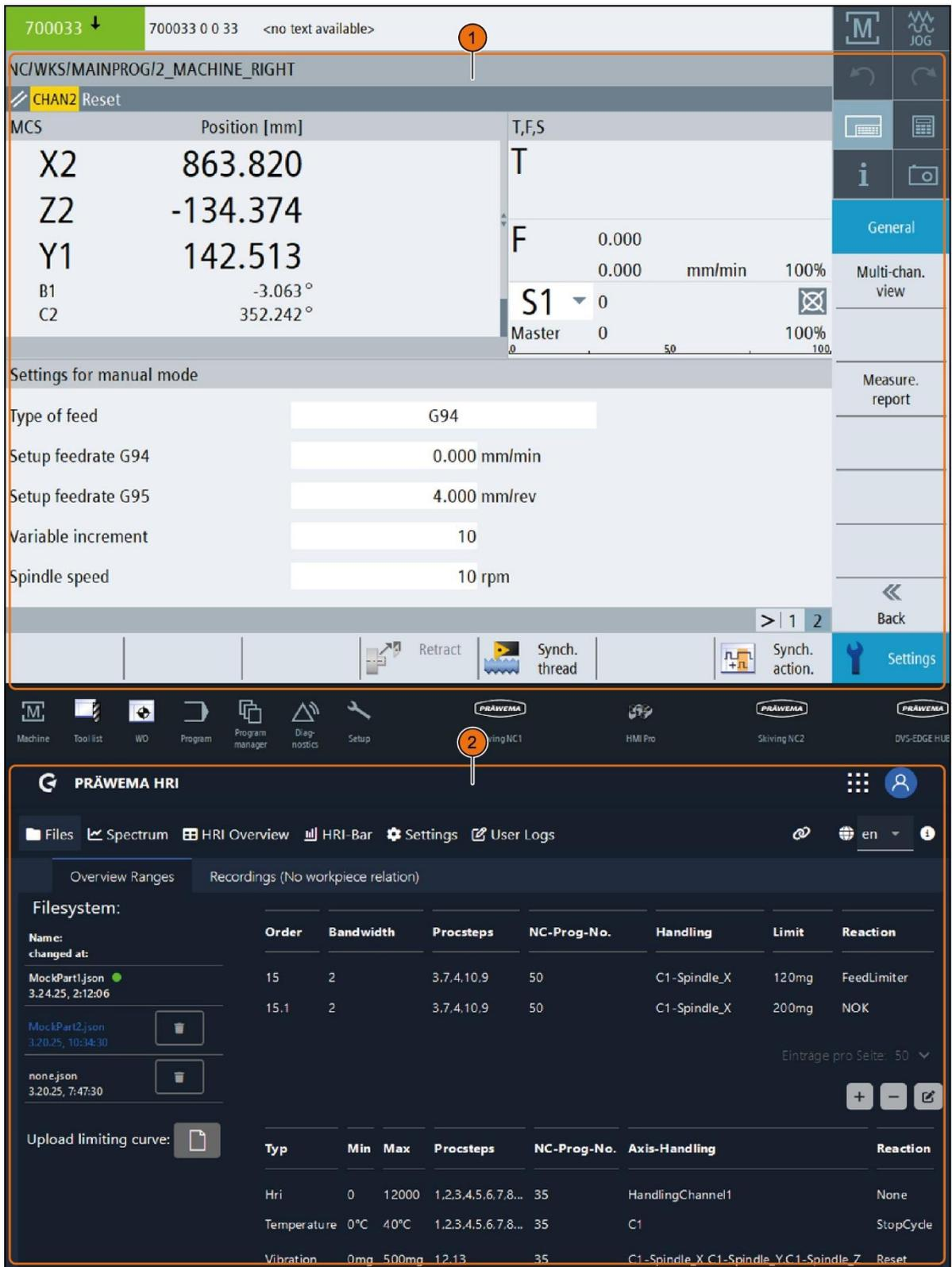
Fig. 122 Display HMI/HRI menu with SynchroForm machines with vertical display
