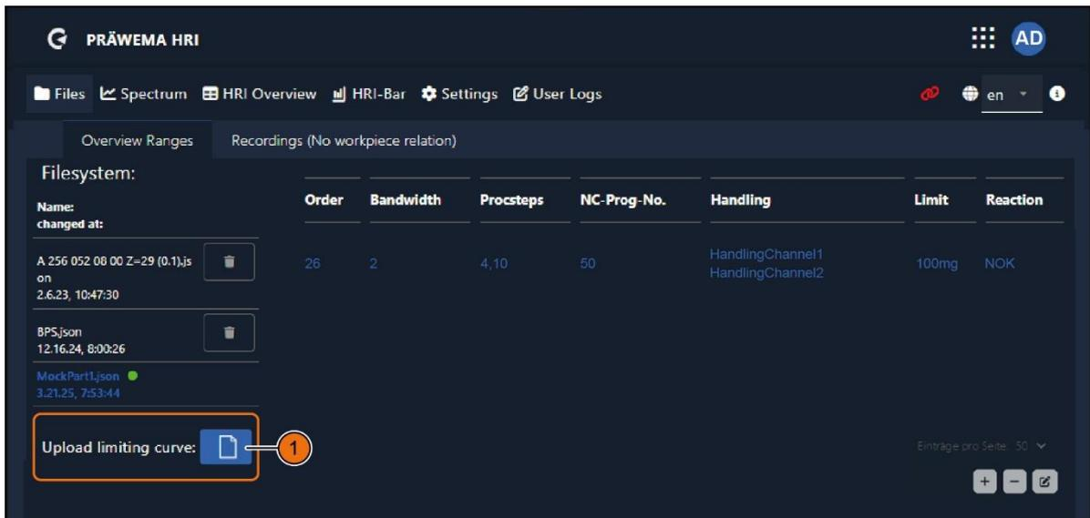
Fig. 55 Files menu - Upload limit curve
