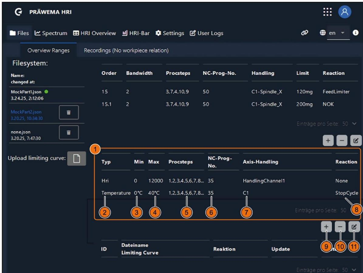
Fig. 13 File system menu - lower area, limiting values of diagnostic object
