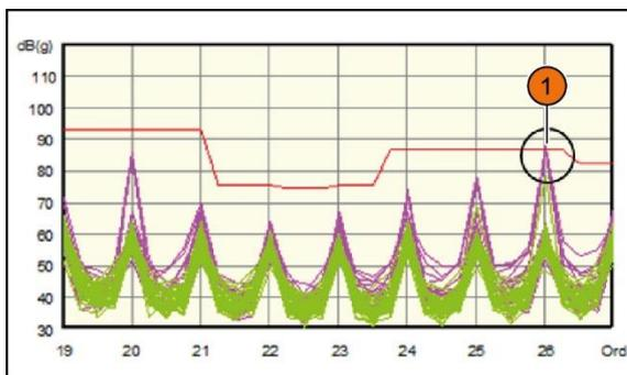
Fig. 54 Result of acoustic test stand
