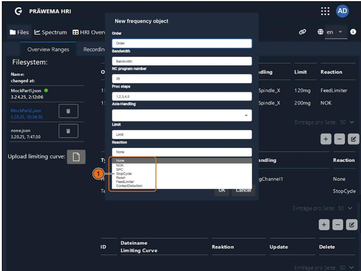
Fig. 52 New frequency object menu - selection list reactions
