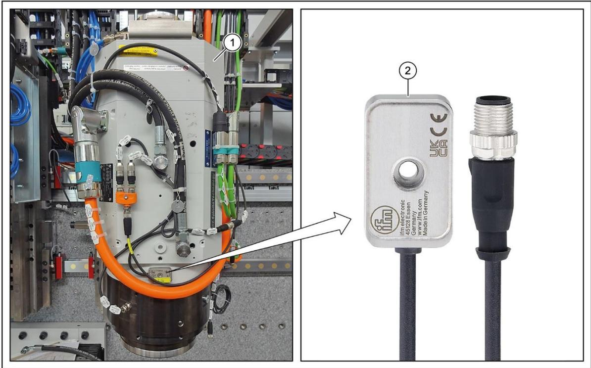
Fig. 120 Vibration sensors on the workpiece spindles - SynchroForm
