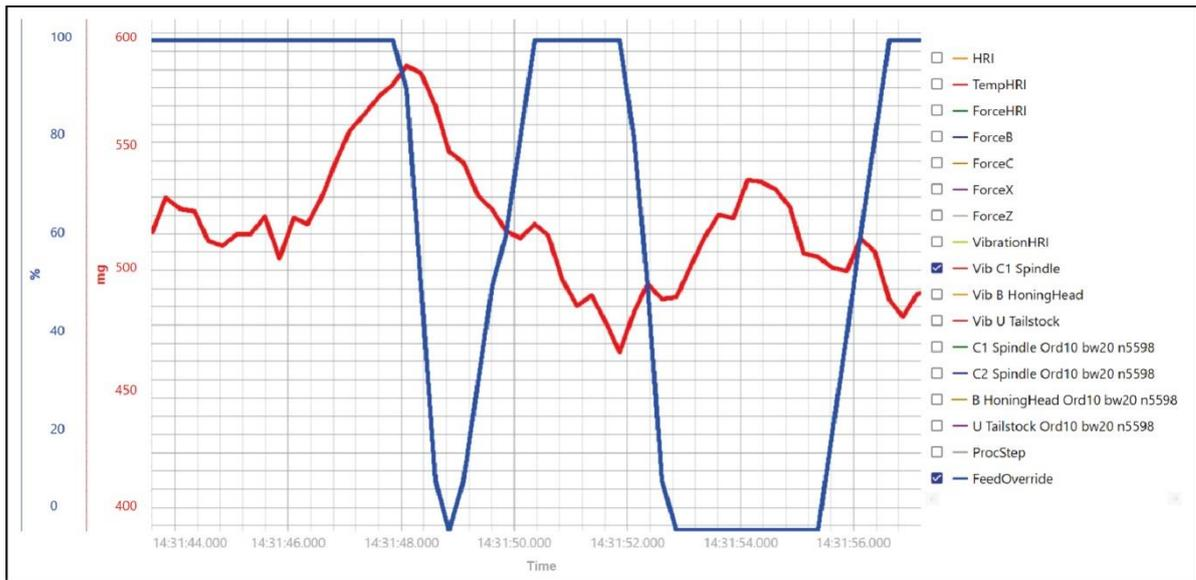
Fig. 23 Example of a feed limitation - feed limiter
