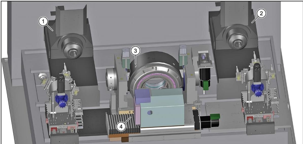
Fig. 106 Overview of vibration sensors on a SynchroFine external honing machine
