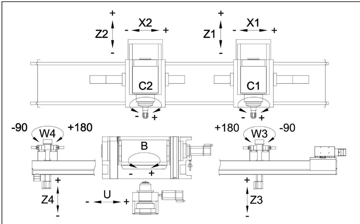
Fig. 100 Axes of a SynchroFine machine
