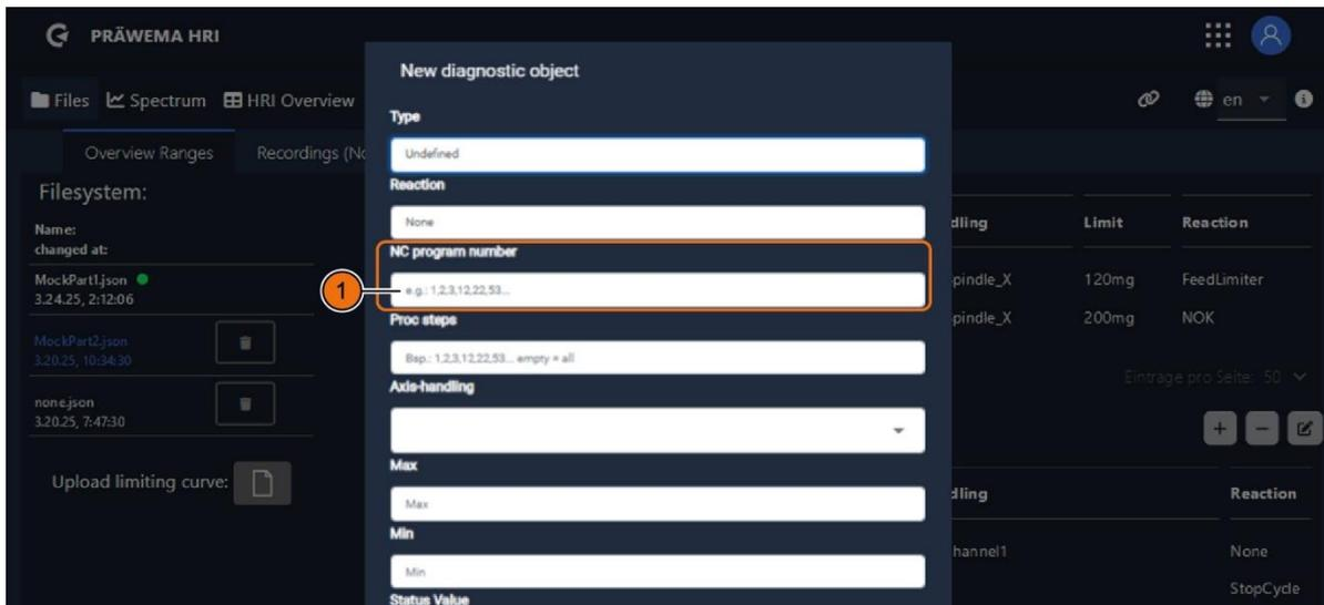
Fig. 17 New Diagnostic object menu - NC-program numbers
