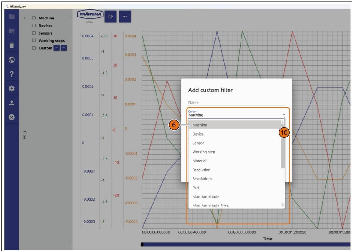
Fig. 82 Add user-defined filter - drop-down menu column
