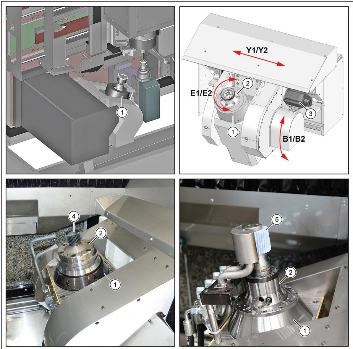
Fig. 115 Tool spindle E1/E2 - skiving modules - SynchroForm (example)
