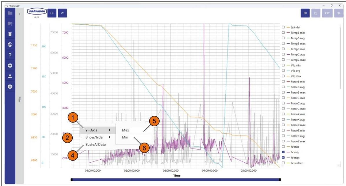
Fig. 78 Dialog field in the line diagram - line 1
