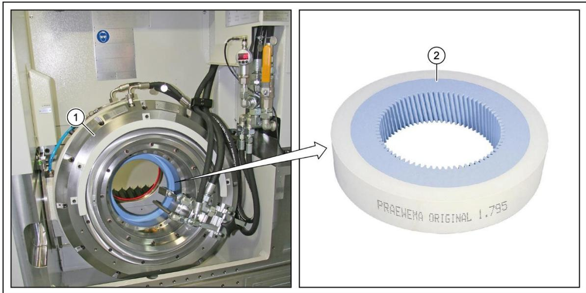
Fig. 103 Honing head with honing tool - SynchroFine
