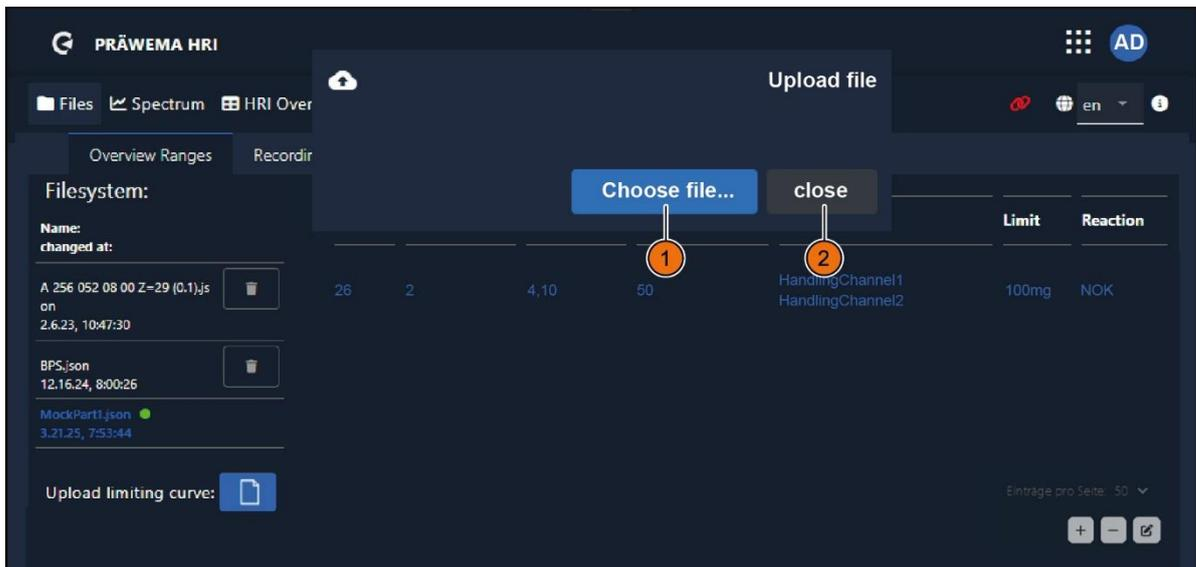
Fig. 56 Files menu - upload limit curve menu window
