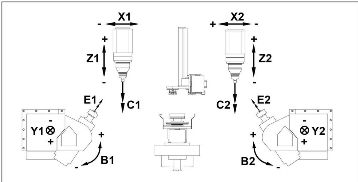
Fig. 113 Axes of a SynchroForm double spindle skiving machine
