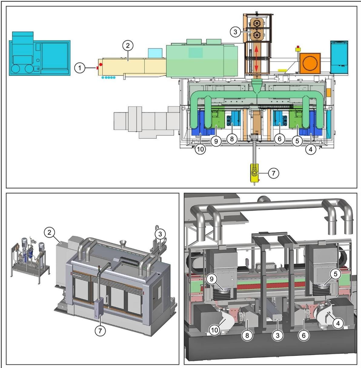
Fig. 114 Module overview of SynchroForm internal honing / skiving machine (example)
