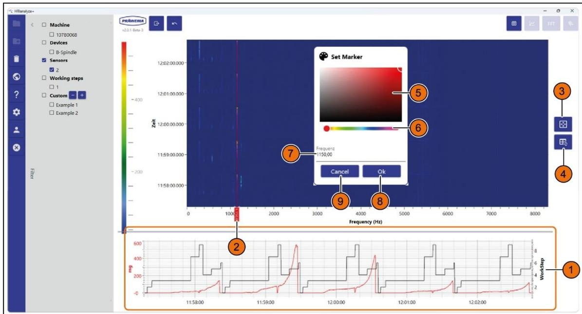
Fig. 89 Dialog field in the Campbell diagram - with line diagram
