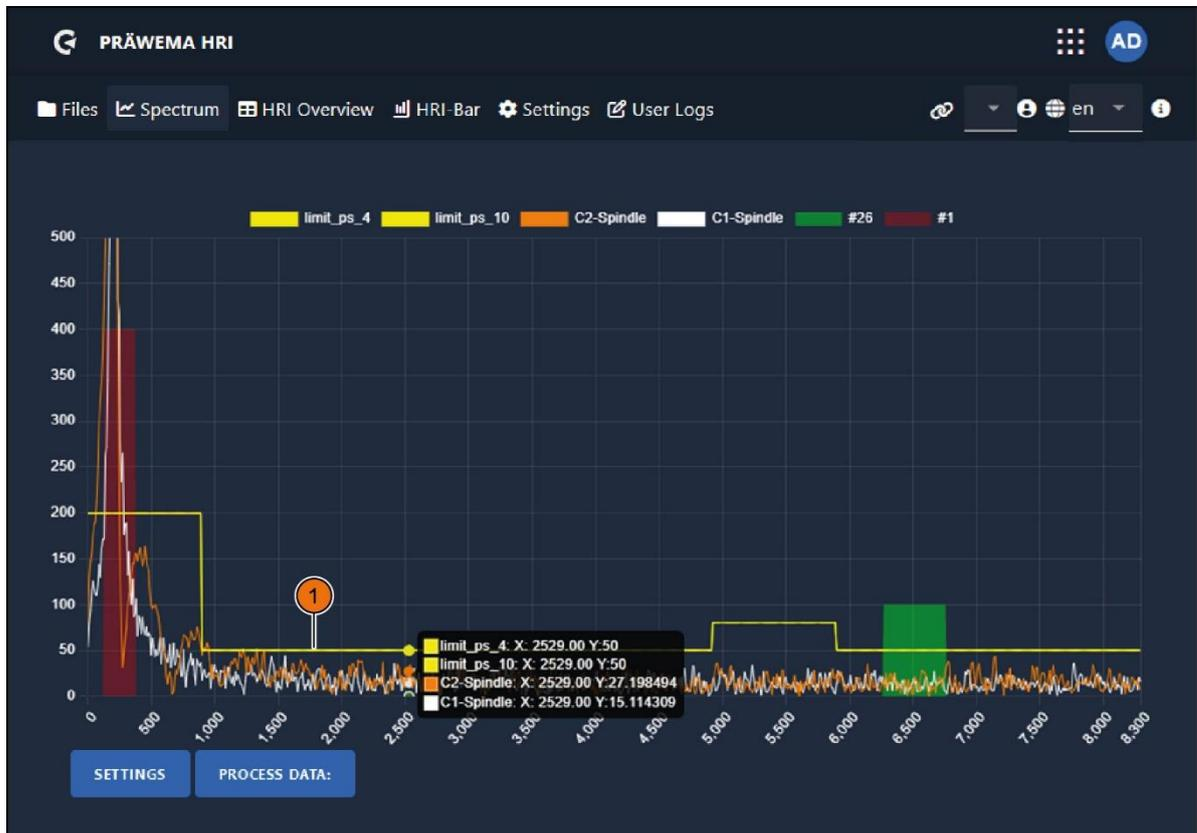
Fig. 64 Spectrum menu - checking the limit curve
