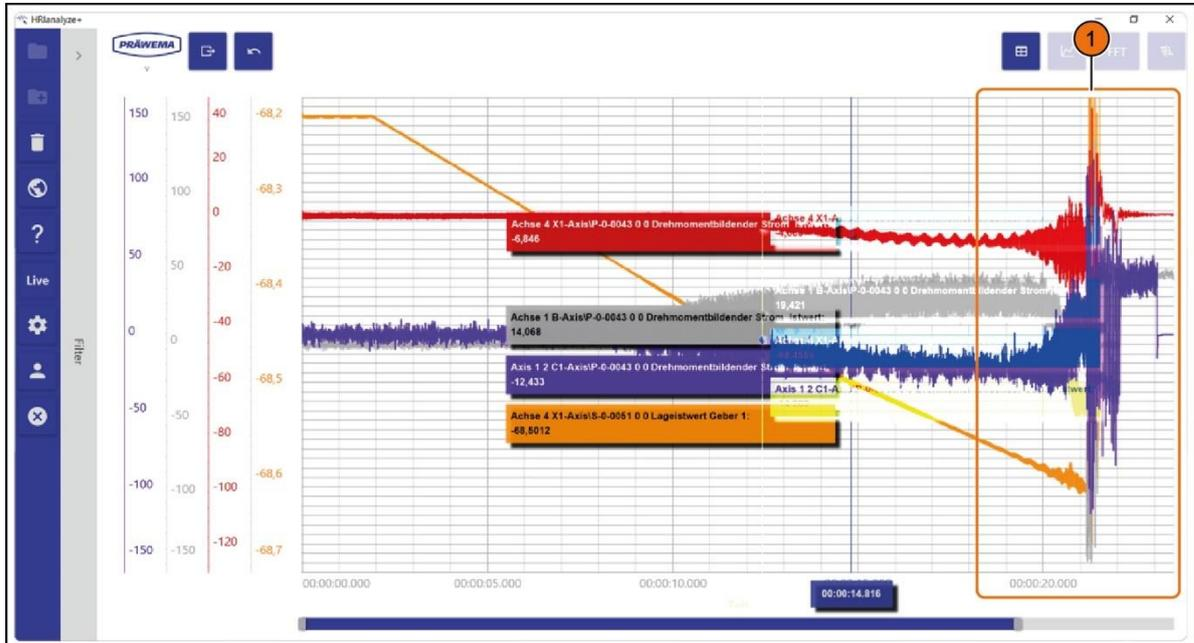
Fig. 99 Example: line diagram - REXROTH INDRA Works - tool breakage
