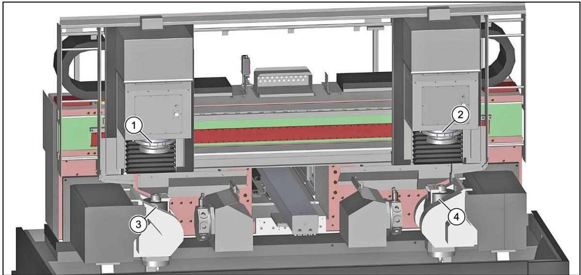
Fig. 117 Overview of vibration sensors skiving machine - SynchroForm
