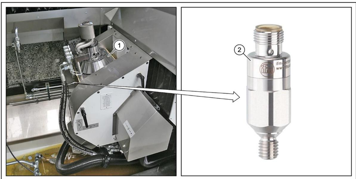
Fig. 119 A single-axis vibration sensor on the tool spindles - SynchroForm
