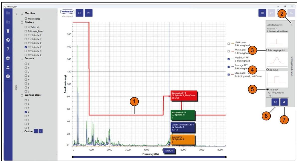
Fig. 92 Fine adjustment of limit curve
