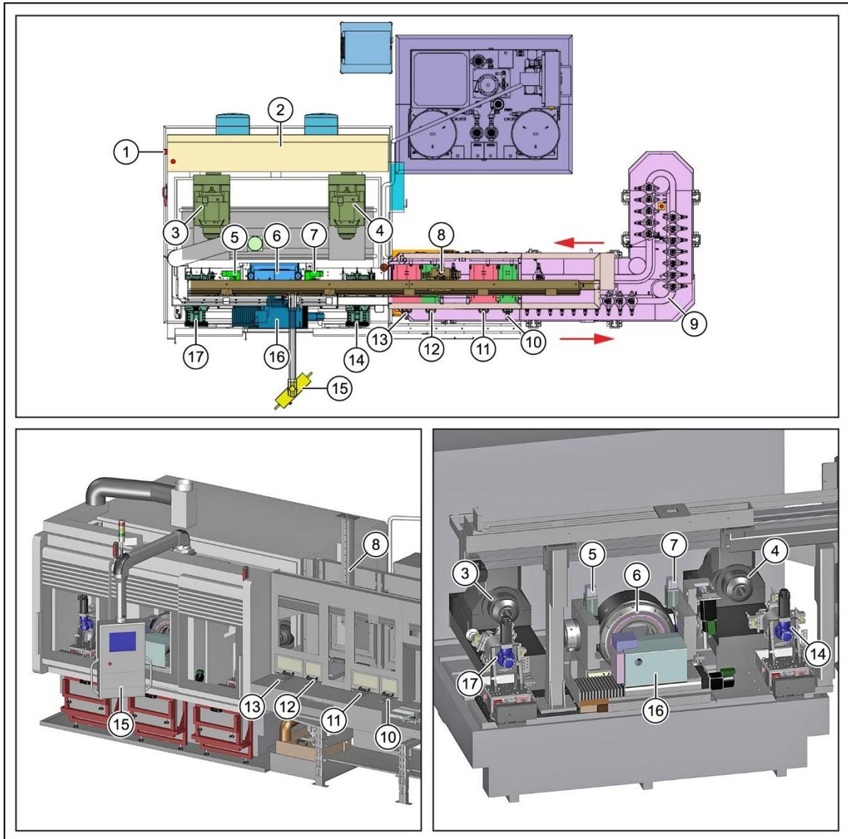
Fig. 101 Module overview, external honing machine SynchroFine (example)
