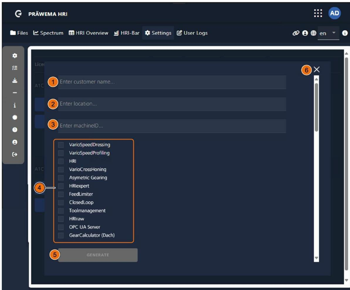
Fig. 43 License management menu - Generate Test license input window
