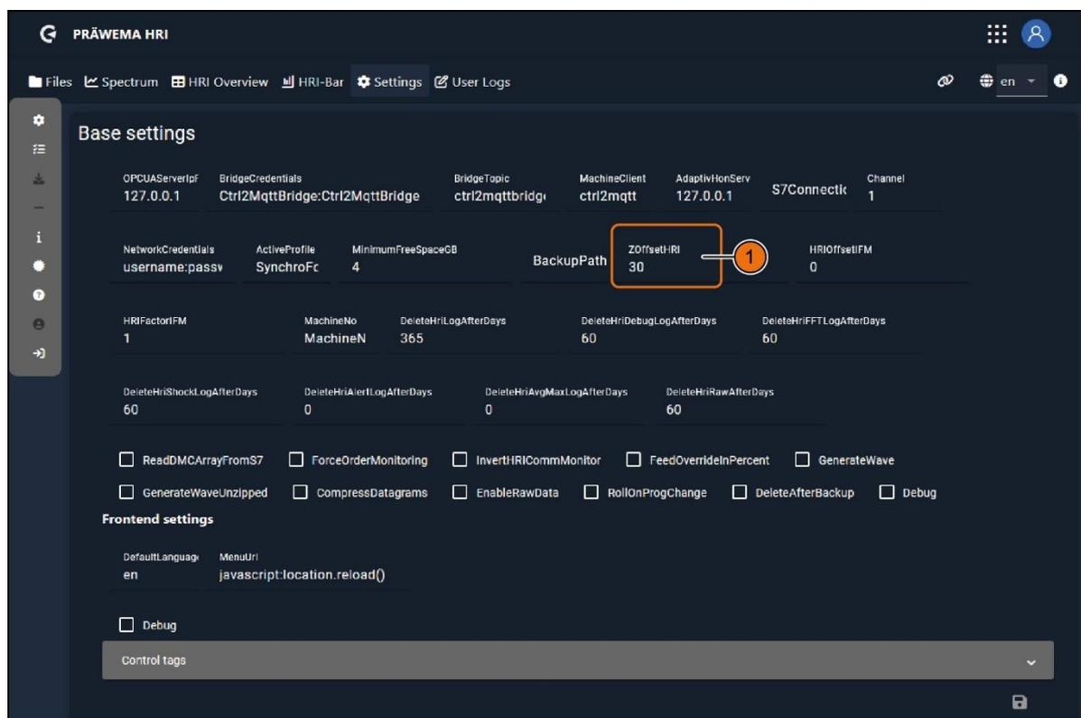
Fig. 6 Basic settings menu - example of setting of the offsets - SynchroFine
