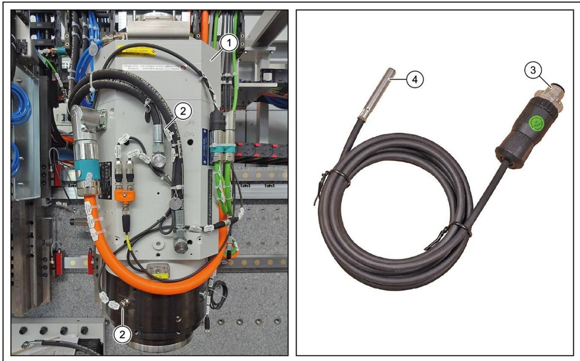
Fig. 121 Temperature sensors on the workpiece spindles - SynchroForm
