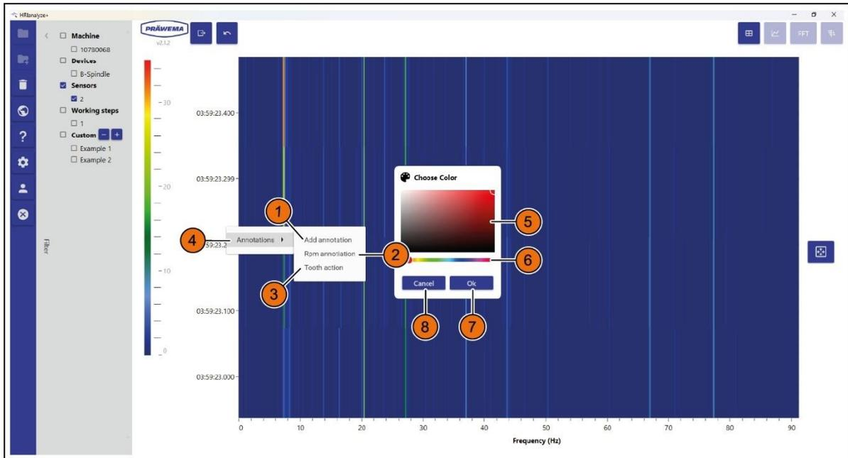
Fig. 88 Dialog field in the Campbell diagram - set marking
