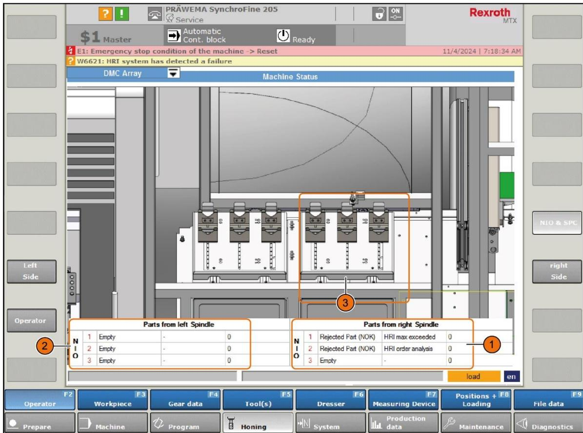
Fig. 21 Status text display in the *HMI menu machine status* (example)
