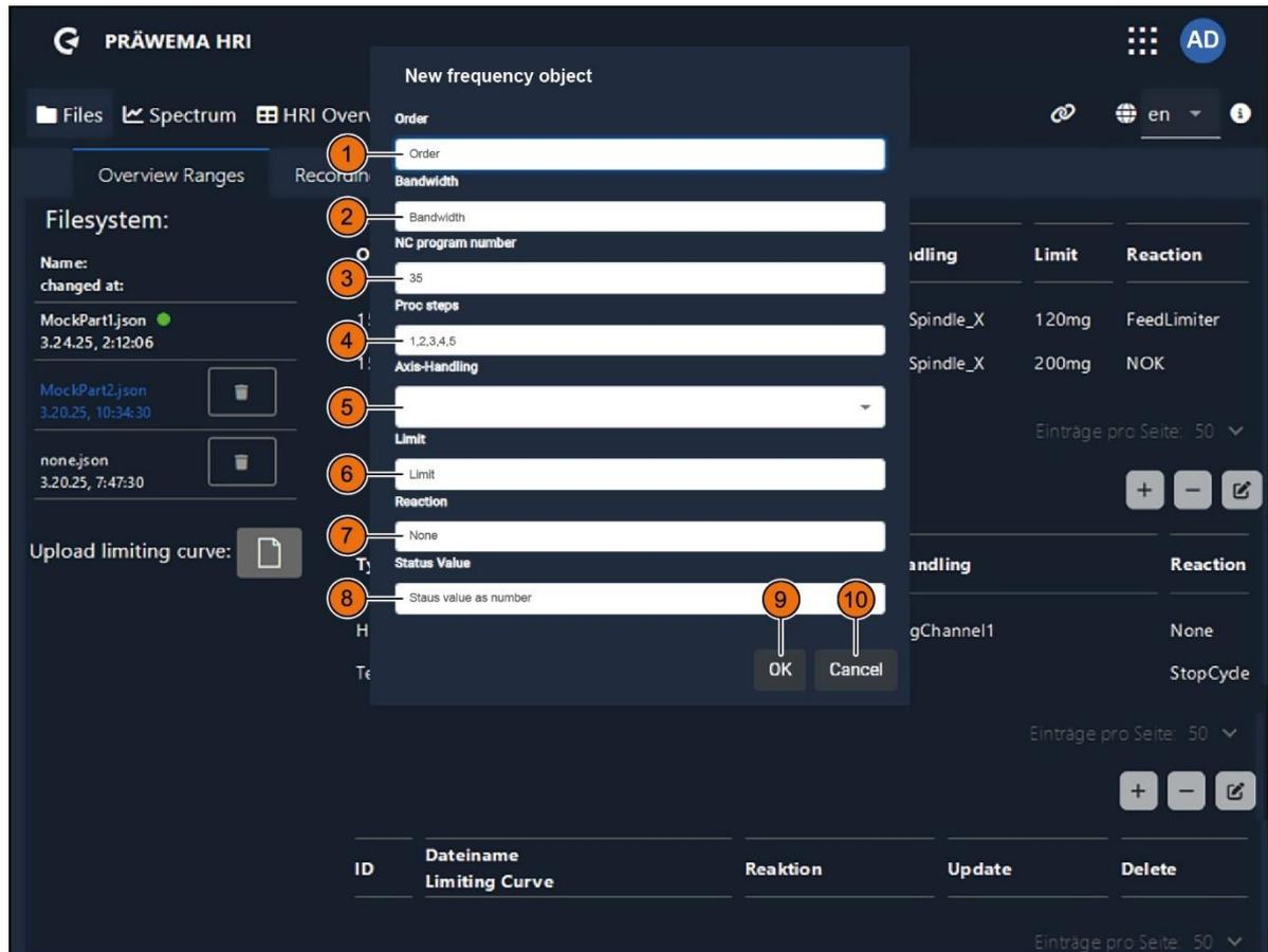
Fig. 51 Input menu: new frequency object
