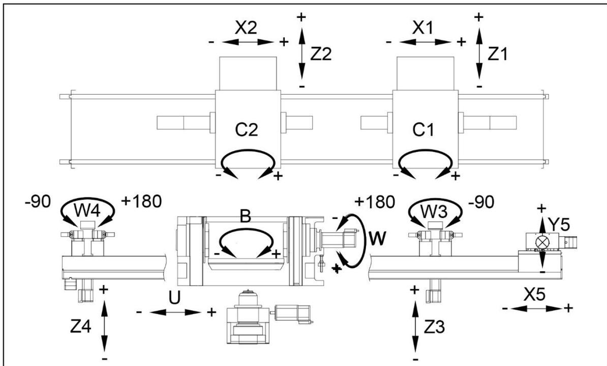
Fig. 105 CNC and positioning axes - SynchroFine
