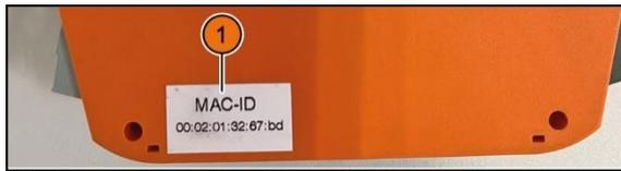
Fig. 35 Adhesive label with MAC address on the VSE evaluation unit
