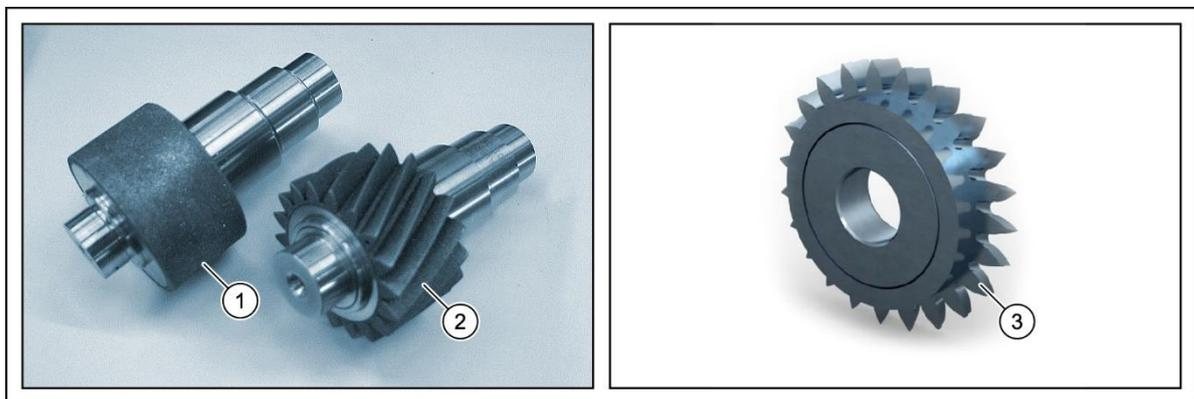
Fig. 104 Dressing tools - SynchroFine
