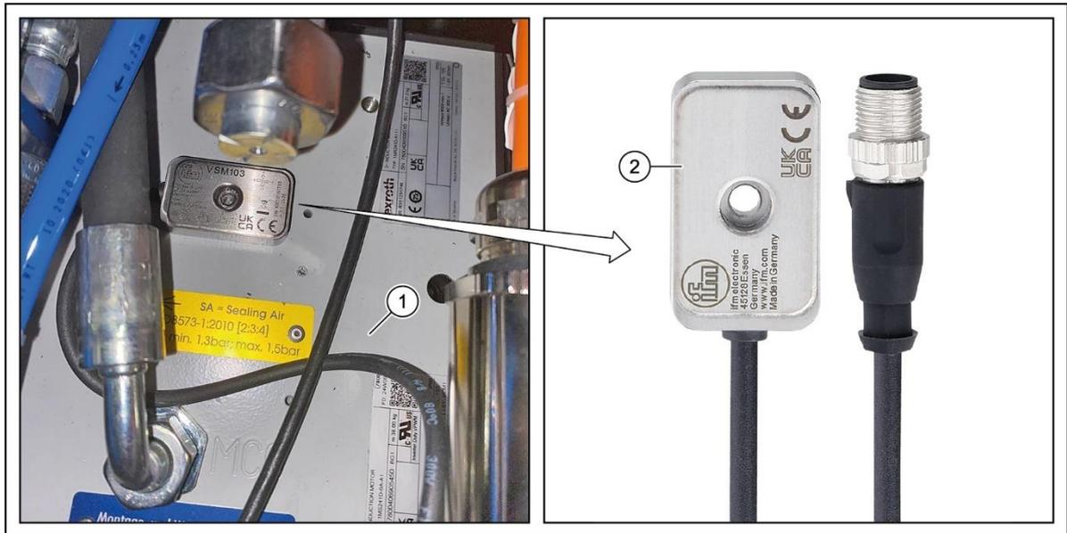
Fig. 108 Vibration sensors on the workpiece spindles - SynchroFine
