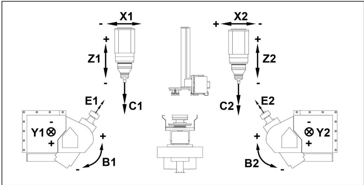
Fig. 116 Axes of the SynchroForm double spindle skiving machine - SynchroForm
