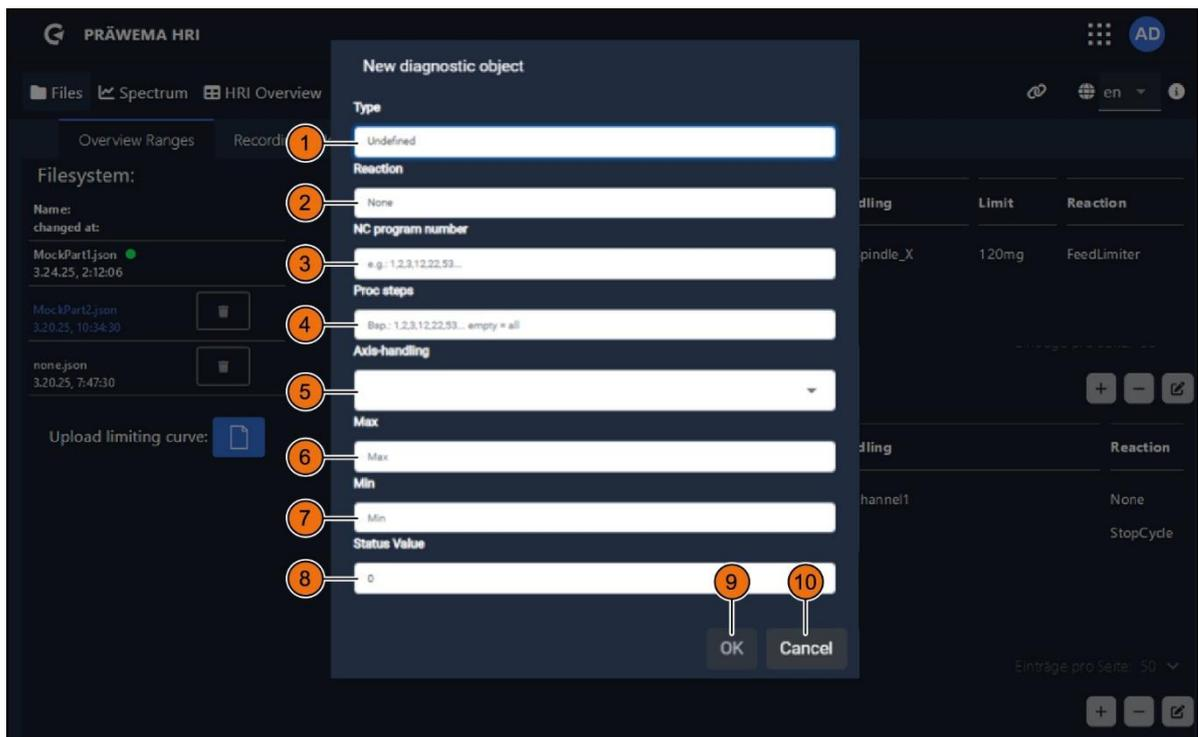
Fig. 14 New diagnostic object - input menu for limiting values
