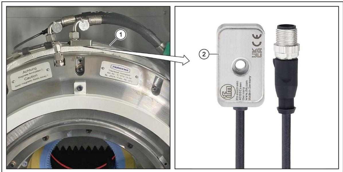
Fig. 109 Vibration sensor on the honing head - SynchroFine
