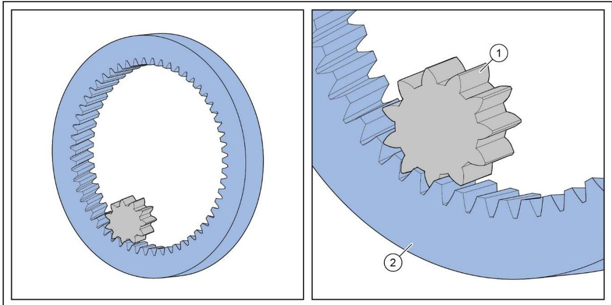
Fig. 102 Model of the honing technology - SynchroFine
