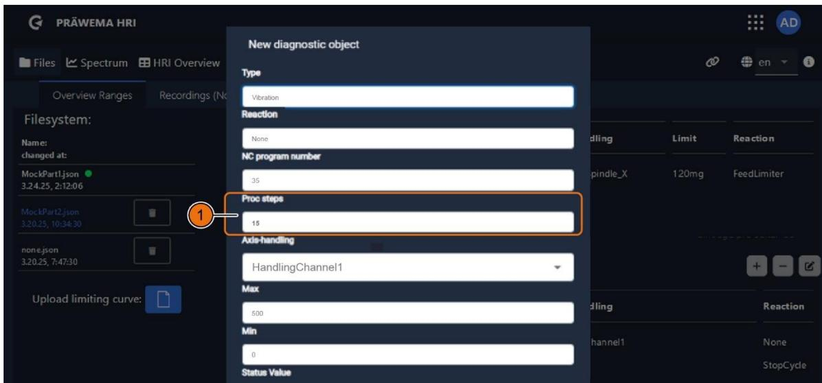
Fig. 19 New diagnostic object menu - program steps of hobbing
