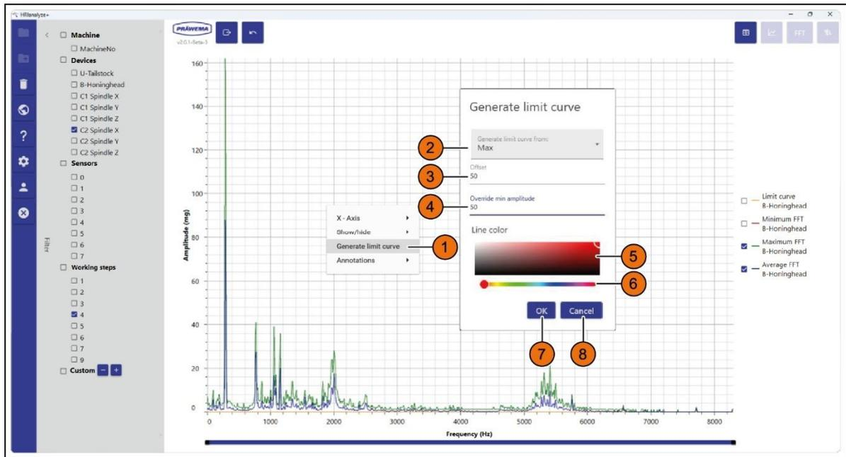
Fig. 90 FFT line diagram - create limit curve
